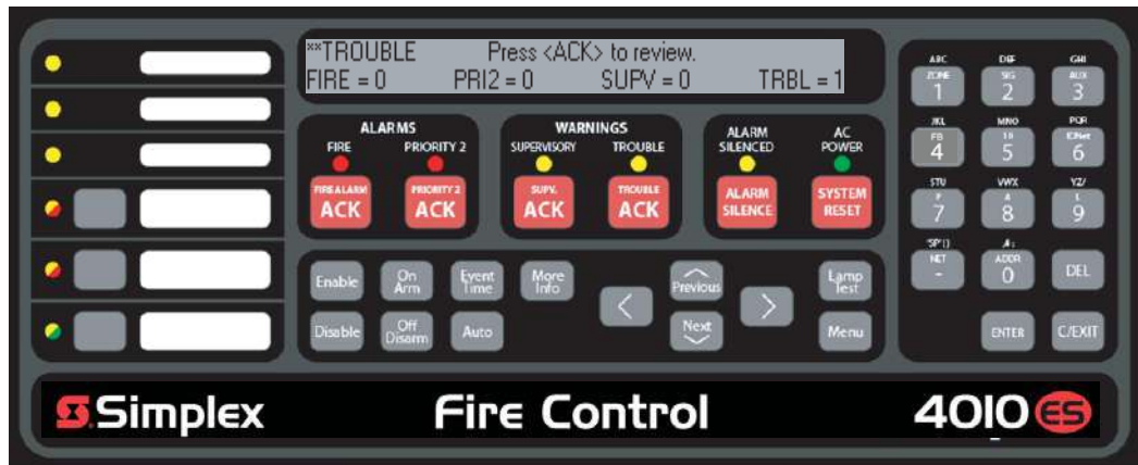
Figure 3-1. Interface Panel Showing Trouble Condition
